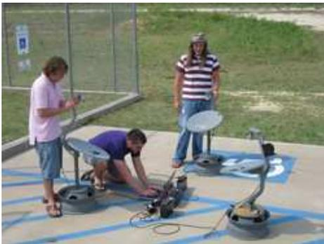
Barr told the ARRL he was initially intrigued by the idea of building a small radio telescope using a cast-off satellite TV antenna and a commercially available satellite signal monitor. "We modified the monitor by adding a small circuit, allowing it to drive a laptop computer's soundcard to gather data and for signal processing. I thought this would be an interesting way to provide hands-on experience for the students here at TSU with tangible results."
