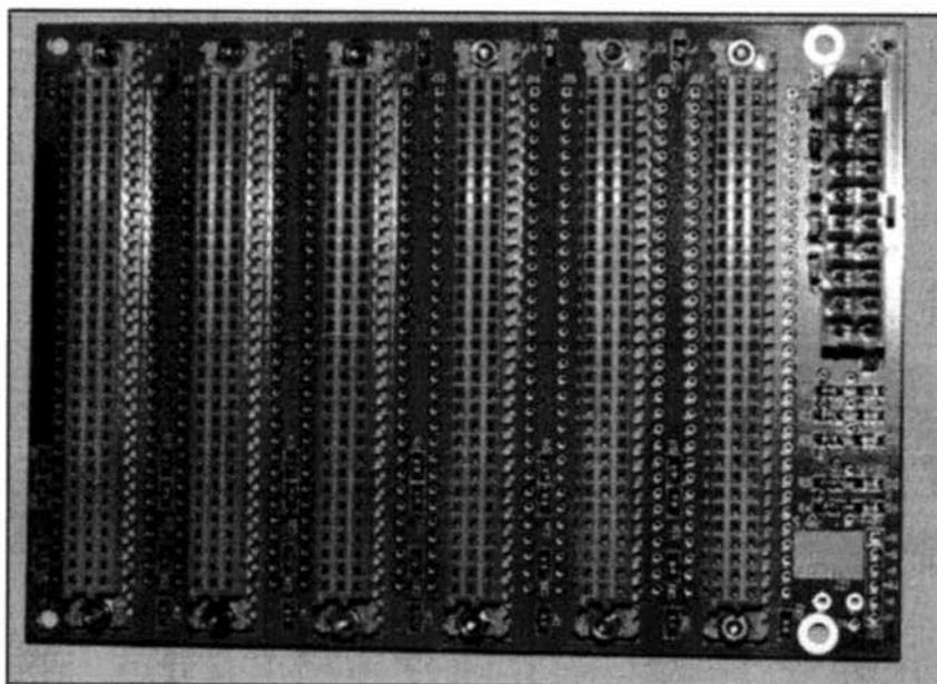
Photo A— The Atlas backplane board, into which all other modules of the OpenHPSDR radio connect. (Photos courtesy the OpenHPSDR Project)
