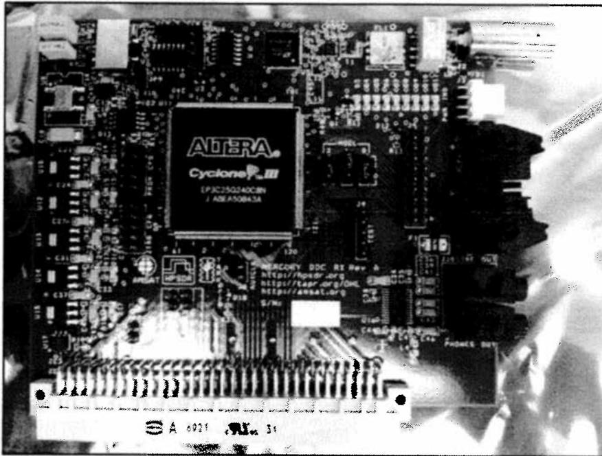
Photo B— An OpenHPSDR Mercury receiver board. The Altera Cyclone FPGA is in the center and the Linear Technologies ADC is at the top center.
