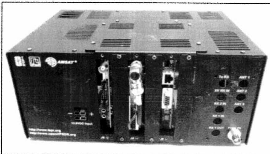
Photo E— An assembled OpenHPSDR transceiver in a Pandora case. The boards are, from left to right: Mercury, Penelope and Metis. Inside the case are an LPU and Pennywhistle (see text for details).
