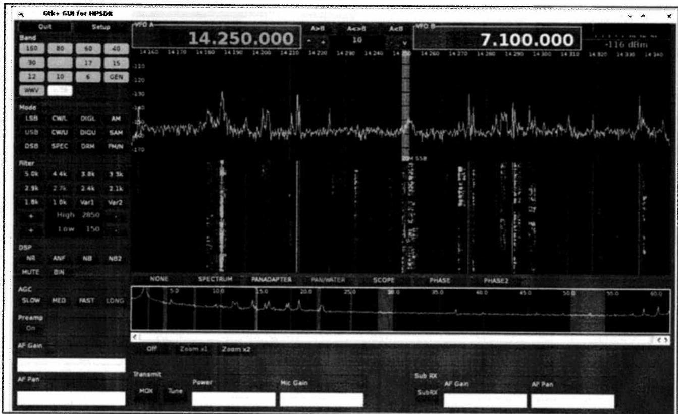
Photo H— GHPSDR is a popular HPSDR program among Linux users. It splits the workload of a software-defined radio into multiple components that can be assembled and run on different computers
